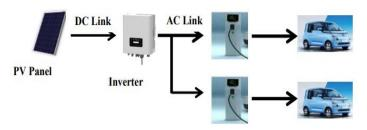
Figure 1: Solar Power EV charging Station diagram
