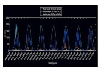
Figure 3: PV Panel Production graph showing peak, median, and minimum weekly output
