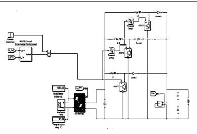
Figure 1: PV to EV Charging subsystem using MPPT
